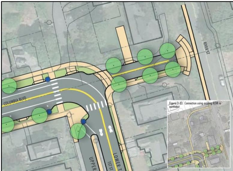
Left: Concept illustrates potential enhancements to the 1st Street/Columbia Blvd. intersection and the overlook area east of the intersection. A bike access trail utilizing existing right-of-way can be seen in the lower right corner.
